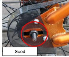
With the original axle nut in place, check both sides of the bike's rear axle to be sure the thread sticks out past the mounting nut at least 3/16" (roughly the thickness of three 0.25¢ coins).
